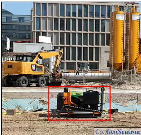
INN – borehole sensors for measurement in cased bores or in drill augers.
