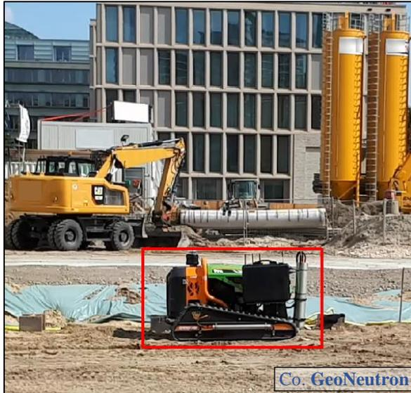
INN - borehole sensor technology for obstacle evaluation behind buildings.
